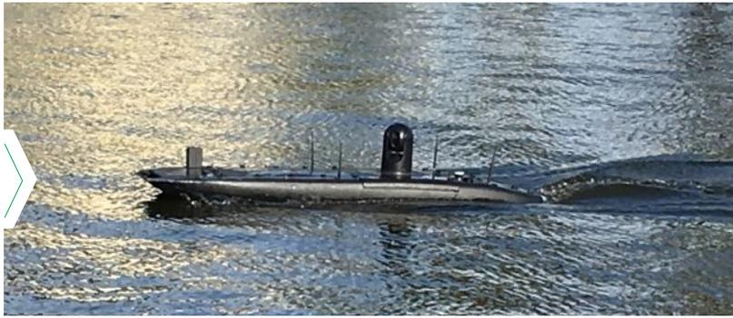
» The MANTAS T-series USVs integrate open-architecture design. The hydrodynamic hull and sleek profile allow higher speeds, with superior maneuverability, while unmanned operation minimizes manpower requirements. Photo credit: Jack Rowley.
